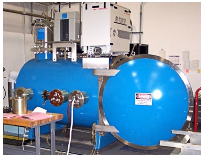
Figure 19: Thermal Vacuum Chamber
