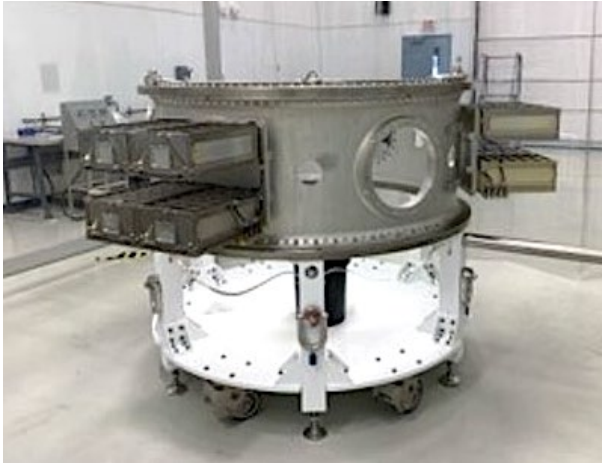
Figure 57: Integrated ESPA ring prior to leaving Wallops (Building F-7)
