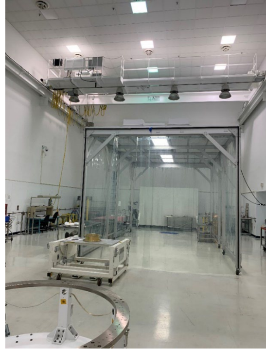
Figure 63: High Bay East Cleanroom Tent with ESPA ring integration ground support equipment in the foreground
