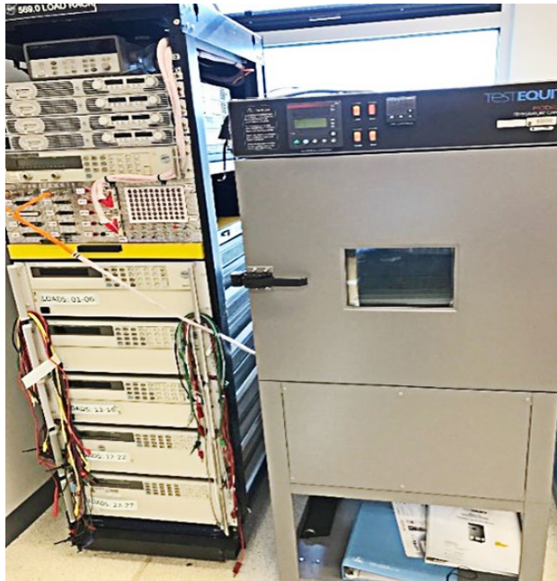
Figure 12: Test Equity Model 115 Thermal Cycle Chamber
